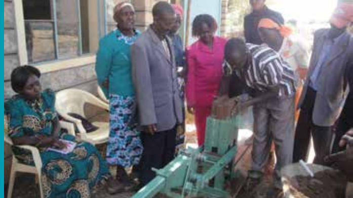
Kikuu Youth Group Members making stabilized soil bricks in Machakos. © Andrew Nyamu
